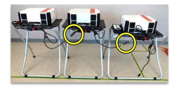
g. Take each Y-Power Cord, fold the cable into a figure-eight, and secure with the Velcro tie. Place four Y-Power Cords into the blue Critical Bag.
