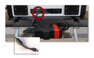
e. Return to the first Duo in the string nearest to the Controller, disconnect the red-taped connector from the red-taped power brick. The red-taped connector is one of the legs of the Y-Power Cord. Continue down the string, disconnecting the red-taped connector from each power brick.
