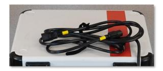
h. The six-foot Power Cord that was connected to the Y-Power Cord and the power strip should be folded together and secured with the Velcro tie. Place the Power Cord into the blue Critical Bag.
