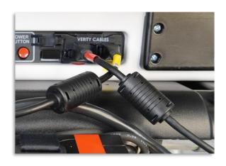
j. After disconnecting the final red-taped Verity Data Cable at the Duo DAU, disconnect the blue USB cable from the back of the Duo. The cable is connected to the ATI Controller. Lift the ATI Controller from the cradle on the Duo DAU Booth Stand. Then, fold the cable and secure it with the Velcro tie. Place the ATI Controller in the blue Critical Bag.
