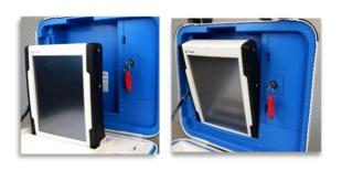
1. Release the lid brace, close the lid, secure the two latches on the front of each Duo and lock with the square key.
