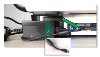
h. Disconnect the Verity Data Cable from the yellow USB port on the back of the Controller. Disconnect the six-foot power cord from the power brick, wrap up the power cables, and secure them with the Velcro ties.
