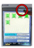
c. Press 'Close Polls' and confirm 'Yes.' Enter the 'Close Polls" password found in the Controller and select 'Accept.' (All Duo tablets will now read 'Closed.') The Controller printer will automatically generate the 'Close Polls Report.'
