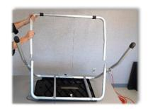
b. Remove the two aluminum leg extensions and the U-shaped aluminum leg brace by depressing the spring-loaded pins.
