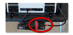
f. Return to the first Duo in the string, disconnect the remaining two yellow-taped connectors of each Y-Power Cord. Continue down the string, disconnecting the yellow-taped connectors as you go.
