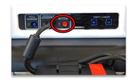
g. Now, disconnect the round connector to the left of the red Power button. The connector is spring-loaded, so grasp it firmly with your thumb on the flat part and your index finger underneath on the round part and pull it free from the unit.
