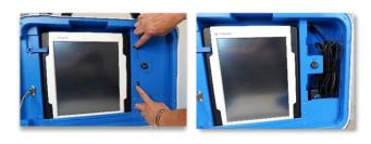
i. Release the lid brace, close the lid, and secure both latches.
