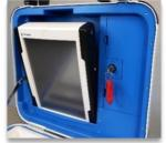
h. Remove the blue panel on the inside of the lid by depressing the latches above and below the lock. Insert the power brick and power cord. Replace the blue panel and secure the latches.
