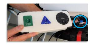
k. Unlock each Duo tablet by turning the key counter-clockwise. Pull the tablet forward from the top, lift it up, and release it from the cradle. Place the tablet in the storage compartment in the lid. Lock the tablet in place by turning the key clockwise. Turn the lever in the upper left-hand corner clockwise to secure the tablet.
