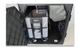
k. While the Ballot Box door is open, reach under the front of the lid. Gently pull the white string down and toward you to release the three locking pins holding the Scan unit to the Ballot Box.
