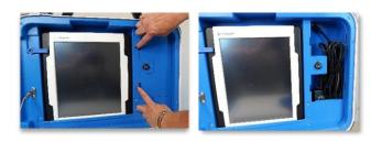
Release the lid brace, close the lid, and secure both latches. Attach the white Controller return seal around the handles. The Controller is now ready for transport by the Election Judge.
