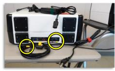
i. Disconnect the Auto Ballot Scanner (scanner gun) USB cable from the white cover above the printer. Wrap up the cable and secure it with the Velcro tie. Place the Auto Ballot Scanner in the blue Critical Bag.
