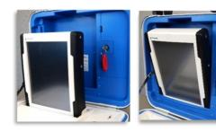
k. Remove the blue panel on the inside of the lid by depressing the latches above and below the lock. Remove the two white return seals and any blue or other unused seals from the compartment. Insert the power brick and power cord. Replace the blue panel and secure the latches.
